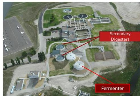
report and used as the foundation for the future fermenter rehabilitation project. The fermenter is a critical component of the biological treatment process. Volatile Fatty Acids (VFAs) created in the fermentation process are used in the Bioreactors to assist microorganisms in nutrient removal. After startup, it takes ~ 2-3 week for the fermenter to create enough VFAs needed to support the treatment process.
